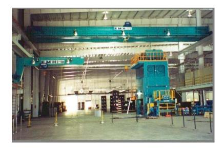
The wall traveling 5 ton crane maximized the use of floor space under the crane by keeping the crane rail off the floor.
