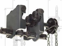
R&M trolleys are designed for both manual and electric operated hoists with a top hook suspension. Both the RPT push trolley and RPTC hand geared trolley are easily adjustable for a wide range of flange widths. Our RPTs are available in 1/4 - 5 ton (250 - 5000 kg) capacities, and the RPTCs are available in 1 - 10 ton (100 - 10,000 kg) capacities.
